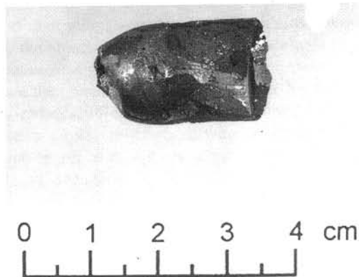
Fig. 1. Picture of typical ingot. Starting charge composition Cu(In 0.8 Ga 0.2 ) 3 Se 5 .
