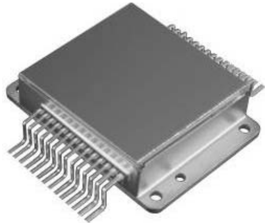
Fig. 6. UL 03 04 1 – 384×288 (320×240), 35- \mu m pixel pitch.
