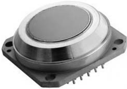
Fig. 4. UL 03 08 1 – 384×288, 35- \mu m pixel pitch.
